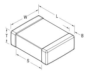
**General Information** Series SMD Auto X7R VW80808 SMD Chip Style Description SMD, MLCC, Automotive Grade Features VW 80808 Specification Compliant RoHS Yes **Flexible Termination** Termination Failure Rate N/A AEC-Q200 Qualifications AEC-Q200 Yes **Typical Component Weight** 21 mg Shelf Life 152 Weeks
