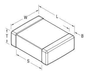
**General Information** Series SMD Auto X7R VW80808 SMD Chip Style Description SMD, MLCC, Automotive Grade Features VW 80808 Specification Compliant RoHS Yes **Flexible Termination** Termination Failure Rate N/A AEC-Q200 Qualifications AEC-Q200 Yes **Typical Component Weight** 25 mg Shelf Life 152 Weeks
