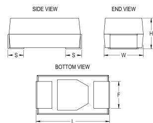
Dielectric Polymer Aluminum Style SMD Chip Description Surface Mount, Polymer Aluminum RoHS Yes Termination Tin Qualifications UL94V-0 AEC-Q200 No Halogen Free Yes Typical Component Weight 305.03 mg 104 Weeks Shelf Life MSL 3
