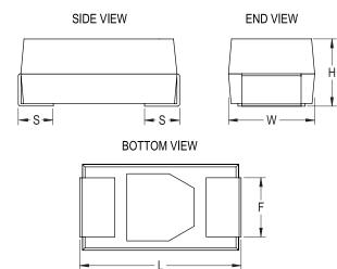
A700 Series Dielectric Polymer Aluminum Style SMD Chip Description Surface Mount, Polymer Aluminum RoHS Yes Termination Tin Qualifications UL94V-0 AEC-Q200 No Halogen Free Yes Typical Component Weight 305.03 mg Shelf Life 104 Weeks MSL 3
