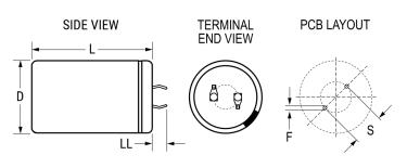
General Information Series ALC70 Dielectric Aluminum Electrolytic Style Snap-In Description Snap-In, Aluminum Electrolytic RoHS Yes Lead 2 Pin AEC-Q200 No Halogen Free true Typical Component Weight 50 g Dimensions D And L Include Sleeving. Notes Shelf Life 156 Weeks
