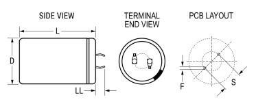
General Information Series ALC70 Dielectric Aluminum Electrolytic Style Snap-In Description Snap-In, Aluminum Electrolytic RoHS Yes Lead 2 Pin Short AEC-Q200 No Halogen Free true Typical Component Weight 28 g Dimensions D And L Include Sleeving. Notes Shelf Life 156 Weeks
