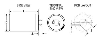
General Information Series ALC80 Dielectric Aluminum Electrolytic Style Snap-In Description Snap-In, Aluminum Electrolytic RoHS Yes Lead 2 Pin Short AEC-Q200 No Halogen Free true Typical Component Weight 60 g Dimensions D And L Include Sleeving. Notes Shelf Life 156 Weeks
