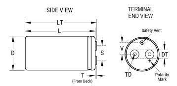
General Information Series ALS30 Dielectric Aluminum Electrolytic Style Screw Terminal Description Screw Terminal, Aluminum Electrolytic RoHS Lead Screw Terminals M5 Mounting Through-Hole AEC-Q200 No **Typical** 90 g Component Weight Dimensions D And L Include Sleeving. MS (MxH) Notes = M8x12. Mounting Clamp (Sold Separately): V3/H2/2736 Shelf Life 156 Weeks
