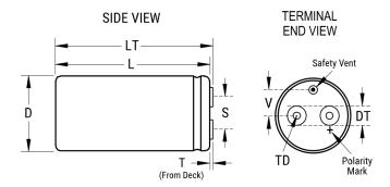
General Information Series ALS30 Dielectric Aluminum Electrolytic Style Screw Terminal Description Screw Terminal, Aluminum Electrolytic RoHS Screw Terminals M5 Lead Mounting Through-Hole AEC-Q200 No **Typical** 140 g Component Weight Dimensions D And L Include Sleeving. MS (MxH) Notes = M8x12. Mounting Clamp (Sold Separately): V3/H2/2736 Shelf Life 156 Weeks
