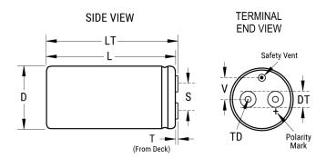
General Information Series ALS36 Dielectric Aluminum Electrolytic Style Screw Terminal Description Screw Terminal, Aluminum Electrolytic RoHS Lead Screw Terminals 1/4-28 UNF 2B Mounting Through-Hole AEC-Q200 No **Typical** Component 1281 g Weight Add 0.015 in/ 0.4 mm to D and 0.045 in/ 1.1 mm to L for Sleeving. Dimension LT Available On Request. MS (MxH) = M12x16. Mounting Clamp Notes (Sold Separately): V11 Shelf Life 156 Weeks
