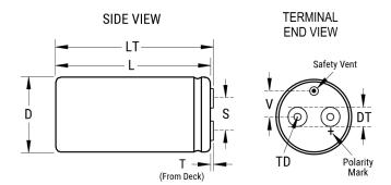
General Information Series ALS36 Dielectric Aluminum Electrolytic Style Screw Terminal Description Screw Terminal, Aluminum Electrolytic RoHS Screw Terminals M6 Lead Mounting Through-Hole AEC-Q200 No **Typical** Component 661 g Weight Add 0.015 in/ 0.4 mm to D and 0.045 in/ 1.1 mm to L for Sleeving. Dimension LT Available On Request. MS (MxH) = M12x16. Mounting Clamp Notes (Sold Separately): V8 Shelf Life 156 Weeks
