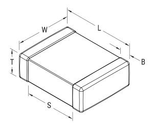
**General Information** Series SMD Auto X7R VW80808 Style SMD Chip Description SMD, MLCC, Automotive Grade VW 80808 Specification Features Compliant RoHS Yes Termination **Flexible Termination** Failure Rate N/A AEC-Q200 Qualifications AEC-Q200 Yes **Typical Component Weight** 7.3 mg Shelf Life 152 Weeks
