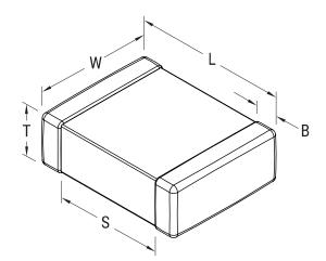
Series SMD Auto X7R HV VW80808 Style SMD Chip Description SMD, MLCC, Automotive Grade VW 80808 Specification Features Compliant RoHS Yes Termination **Flexible Termination** Failure Rate N/A AEC-Q200 Qualifications AEC-Q200 Yes **Typical Component Weight** 21 mg Shelf Life 152 Weeks
