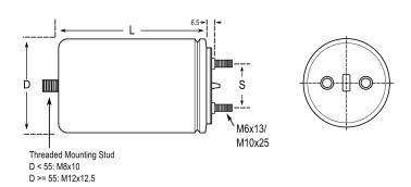
**General Information** Series C44A Dielectric Metallized Polypropylene Style RoHS With Exemptions **REACH** SVHC (Pb - CAS 7439-92-1) cc1c1ec4-db9e-4815-b26b-SCIP Number e8a34ddfb776 Lead Threaded Studs M6 AEC-Q200 No **Typical Component** 441.7 g Weight Miscellaneous Thermal Resistance = 8 C/W.
