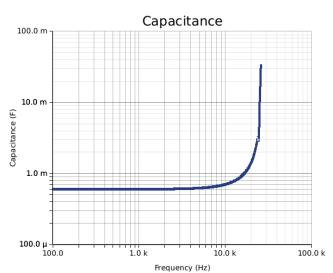
C44U, Film, Metallized Polypropylene, DC Link, 600 uF, 10%, 900 VDC,
