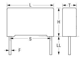
**General Information** C4AQ-P Series Dielectric Metallized Polypropylene Style Radial Features DC Filtering RoHS Yes Lead Wire Leads Qualifications AEC-Q200, IEC61071, EN61071, VDE0560 AEC-Q200 Yes 15.7 g Typical Component Weight Rth = 36 C/W. Miscellaneous
