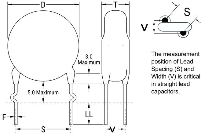
The measurement position of Lead Spacing (S) and Width (V) is critical in straight lead capacitors.
