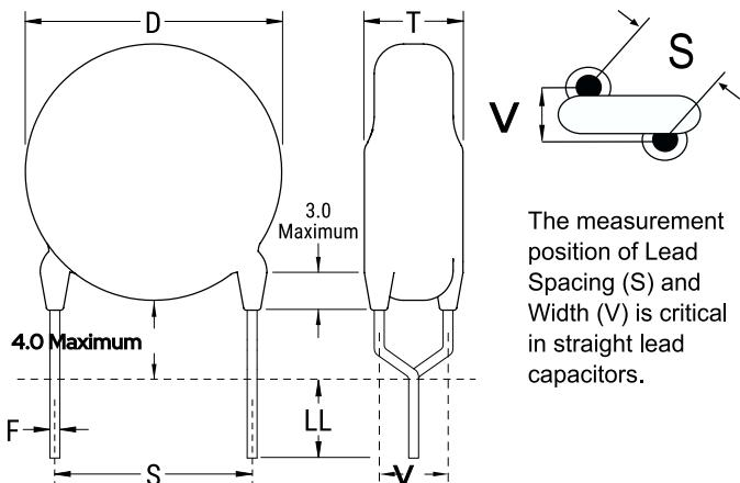
The measurement position of Lead Spacing (S) and Width (V) is critical in straight lead capacitors.
