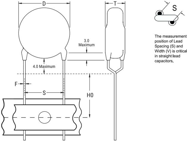
The measurement position of Lead Spacing (S) and Width (V) is critical in straight lead capacitors.
