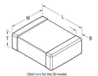
SMD Chip Style Description SMD, Fixed, RF, Ultra High Q, Low ESR, Class I Features Ultra High Q, Low ESR, Class I RoHS Yes Termination Tin Marking No AEC-Q200 No Typical Component Weight 0.3 mg Notes Solder Reflow Only. Shelf Life 78 Weeks MSL 1
