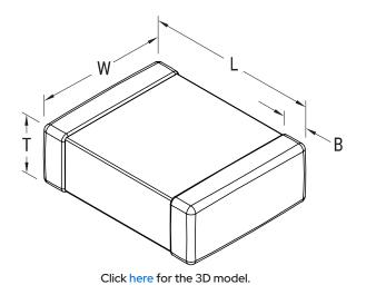
Description SMD, Fixed, RF, Ultra High Q, Low ESR, Class I Features Ultra High Q, Low ESR, Class I RoHS Yes Termination Tin Marking No AEC-Q200 No 1.37 mg Typical Component Weight Notes Solder Reflow Only. Shelf Life 78 Weeks MSL 1
