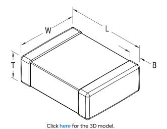
CBR-SMD RF COG Series SMD Chip Style Description SMD, Fixed, RF, Ultra High Q, Low ESR, Class I Features Ultra High Q, Low ESR, Class I RoHS Yes Termination Tin Marking No AEC-Q200 No Typical Component Weight 5.29 mg Notes Solder Wave or Solder Reflow. Shelf Life 78 Weeks MSL 1
