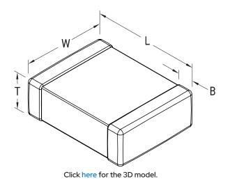
Style SMD Chip Description SMD, Fixed, RF, Ultra High Q, Low ESR, Class I Features Ultra High Q, Low ESR, Class I RoHS Yes Termination Tin Marking No AEC-Q200 No 12.03 mg Typical Component Weight Notes Solder Wave or Solder Reflow. Shelf Life 78 Weeks MSL 1
