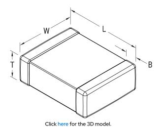
Description SMD, Fixed, RF, Ultra High Q, Low ESR, Class I Features Ultra High Q, Low ESR, Class I RoHS Yes Termination Tin Marking No AEC-Q200 No Typical Component Weight 12.03 mg Notes Solder Wave or Solder Reflow. Shelf Life 78 Weeks MSL 1
