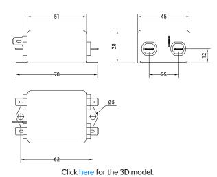
FLLE2-Q Series Style **Chassis Mount** Description Single Phase, Chassis Mount Filters Features Single Phase Phase Single-phase RoHS Yes Qualifications IEC/EN 60939, UL, CSA AEC-Q200 No Lead Fast On **Terminal Type** Faston Test Voltage DC (P to N) 1300 VDC
