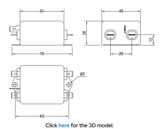
**General Information** FLLE2-Q Series Style **Chassis Mount** Description Single Phase, Chassis Mount Filters Features Single Phase, Medical Phase Single-phase RoHS Yes Qualifications IEC/EN 60939, UL, CSA AEC-Q200 No Lead Wire Leads **Terminal Type** Wire Test Voltage DC (P to N) 1300 VDC
