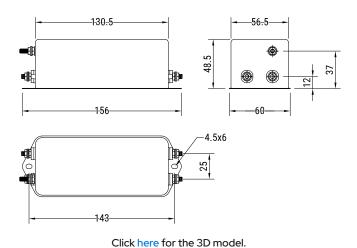
FLLE2-U Series **Chassis Mount** Style Description Single Phase, Chassis Mount Filters Features Single Phase Phase Single-phase RoHS Yes Qualifications IEC/EN 60939, UL, CSA AEC-Q200 No Lead Wire Leads **Terminal Type** Wire Test Voltage DC (P to N) 1300 VDC
