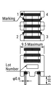
**Pin Pattern Gauge Dimensions - Millimeters**
