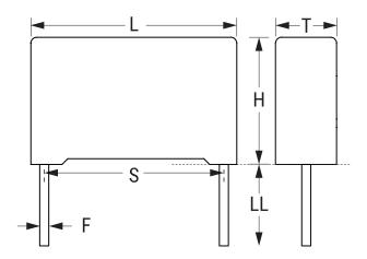
R76 Series Dielectric **Double Metallized** Polypropylene Style Radial Features Pulse RoHS Yes Cut (Tinned Wire) Termination Lead Cut AEC-Q200 No Typical Component Weight 8.45 g
