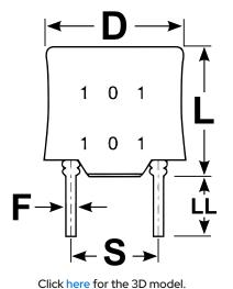
**General Information** SBCP-11HY Series Style Through-Hole Drum Core Ferrite Description Radial Leaded, Ferrite Power Inductors Features DC-DC Converters, Nickel-Zinc (NiZn) Ferrite Core RoHS Yes Wire Leads Lead Contains 4 Reels of 400 pieces Notes each. Do Not Expose To Direct Sunlight.
