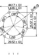
**General Information** SC39XV-S Series Through-Hole Style Features High Impedance, High Rated Voltage RoHS Yes Qualifications AEC-Q200 AEC-Q200 Yes Lead Spacing (S/S1) Are For Reference Only. Notes Miscellaneous Temperature Rise Maximum: 35 Κ. Core Mn-Zn Ferrite
