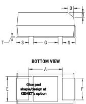
Style SMD Chip Description SMD, MnO2, Molded, Low ESR Features Low ESR RoHS No Prop 65 WARNING: Cancer and reproductive harm https://www.p65warnings.ca.gov SCIP Number 1dd2e1b8-26dd-4d52-927c-6f9 d519011aa Termination Tin Lead (SnPb) AEC-Q200 No Typical Component Weight 446.84 mg Shelf Life 156 Weeks MSL 1
