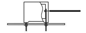
Temperature monitored inside the capacitor.
