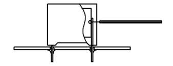
Temperature monitored inside the capacitor.
