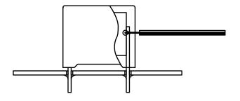
Temperature monitored inside the capacitor.
