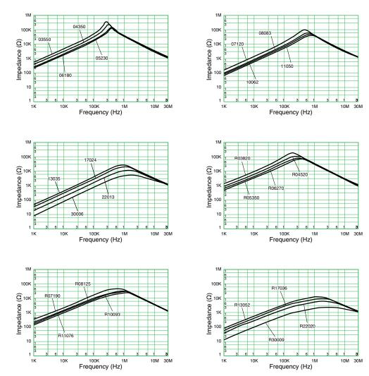
AC Line Filters - Common Mode SS Coils, 11V/H-CH Series
