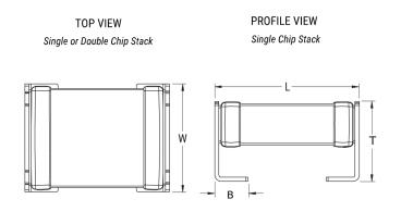
General Information Series KPS SMD Auto X7R Style Stacked Chip SMD, MLCC, Stacked, Single Chip, Class II, Description Automotive Grade Features **Automotive Grade** RoHS Yes Termination Tin Qualifications AEC-Q200 AEC-Q200 Yes **Typical Component** 160 mg Weight Chip Size 1210-1 Shelf Life 78 Weeks MSL
