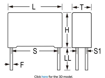
**General Information** C4AK Series Dielectric Metallized Polypropylene Style Radial Features DC Filtering RoHS Yes Lead 4 Wire Leads Qualifications AEC-Q200, IEC61071, EN61071, VDE0560 AEC-Q200 Yes **Typical Component Weight** 50 g Rth = 20 C/W. Miscellaneous
