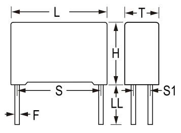
**General Information** C4AQ-P Series Dielectric Metallized Polypropylene Style Radial Features DC Filtering RoHS Yes Lead 4 Wire Leads Qualifications AEC-Q200, IEC61071, EN61071, VDE0560 AEC-Q200 Yes **Typical Component Weight** 104 g Rth = 13 C/W. Miscellaneous
