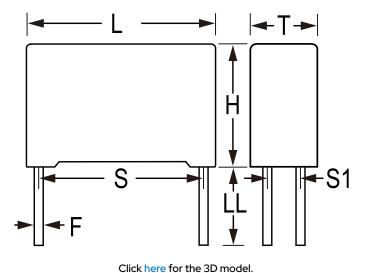
**General Information** C4AQ-P Series Dielectric Metallized Polypropylene Style Radial Features DC Filtering RoHS Yes Lead 4 Wire Leads Qualifications AEC-Q200, IEC61071, EN61071, VDE0560 AEC-Q200 Yes **Typical Component Weight** 193.5 g Rth = 8 C/W. Miscellaneous
