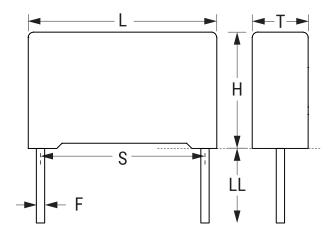
Style Radial Features DC Filtering RoHS Yes Lead Wire Leads Qualifications AEC-Q200, IEC61071, EN61071, VDE0560 AEC-Q200 Yes 18 g Typical Component Weight Rth = 39 C/W. Miscellaneous
