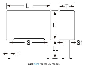
**General Information** C4AU Series Dielectric Metallized Polypropylene Style Radial Features DC Filtering RoHS Yes Lead 4 Wire Leads Qualifications AEC-Q200, IEC61071, EN61071, VDE0560 AEC-Q200 Yes **Typical Component Weight** 64.9 g Rth = 17 C/W. Miscellaneous
