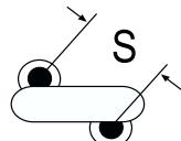
The measurement position of Lead Spacing (S) and Width (V) is critical in straight lead capacitors.
