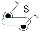
The measurement position of Lead Spacing (S) and Width (V) is critical in straight lead capacitors.
