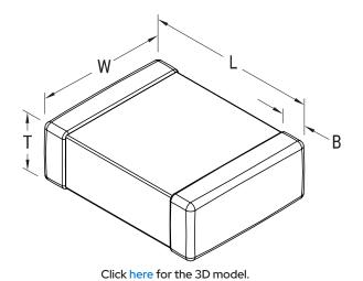
CBR-SMD RF COG Series Style SMD Chip SMD, Fixed, RF, Ultra High Q, Description Low ESR, Class I Features Ultra High Q, Low ESR, Class I RoHS Yes Termination Tin Marking No AEC-Q200 No Typical Component Weight 0.3 mg Notes Solder Reflow Only. Shelf Life 78 Weeks MSL 1
