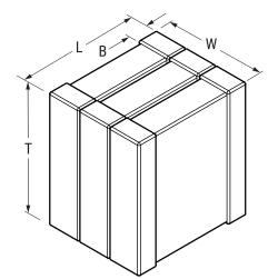
Series KONNEKT KC-LINK Comm COG KONNEKT Style Description KC-LINK with KONNEKT, SMD, MLCC, Ultra-Stable, Class I Features Ultra-Stable RoHS Yes Termination Tin AEC-Q200 No **Typical Component Weight** 3.3 g Notes 3-Chip Low Loss Orientation. 3640-3 Chip Size MSL 1
