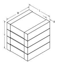
**General Information** Series KONNEKT KC-LINK Comm COG KONNEKT Style Description KC-LINK with KONNEKT, SMD, MLCC, Ultra-Stable, Class I Features Ultra-Stable RoHS Yes Termination Tin AEC-Q200 No 4.3 g **Typical Component Weight** Notes 4-Chip Standard Orientation. Chip Size 3640-4 MSL 1
