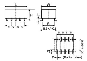
General InformationSeriesEB2StyleSMDDescriptionMiniature Signal Relay, Non-latchFeaturesCompact Size, Flat-Package.<br/>FCC (1500 V) surge capacity. UL<br/>recognized and CSA certified.<br/>Low power consumption<br/>(100-200 mW)RoHSYesCoil TypeSingle Coil (Non-Latching)
