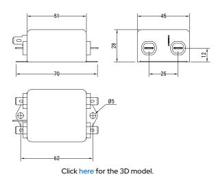
**General Information** FLLE2-S Series Style **Chassis Mount** Description Single Phase, Chassis Mount Filters Features Single Phase Phase Single-phase RoHS Yes Qualifications IEC/EN 60939, UL, CSA AEC-Q200 No Lead Fast On **Terminal Type** Faston Test Voltage DC (P to N) 1300 VDC
