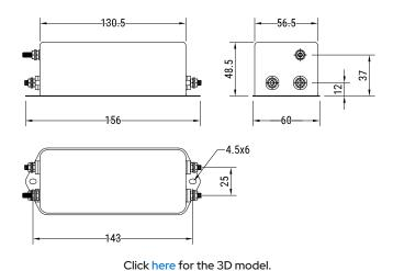
**General Information** FLLE2-U Series **Chassis Mount** Style Description Single Phase, Chassis Mount Filters Single Phase Features Phase Single-phase RoHS Yes Qualifications IEC/EN 60939, UL, CSA AEC-Q200 No Lead Threaded Studs M4 **Terminal Type** Threaded Studs M4 1300 VDC Test Voltage DC (P to N)
